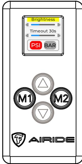
Hold down M1 and M2 to access the passcode entry screen.
