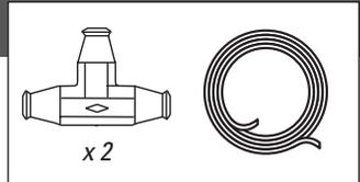
**1** Route the Air Tubing from 1/8 NPT Push-to-Connect Straight Fitting on the top of the Air Compressor to the first 1/4" Push-to-Connect Tee.
