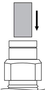
**2** Push Air Tubing into Air Fitting as far as possible.
