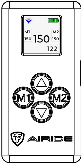
Hold the up and down arrows at the same time to access the remote settings screen.
