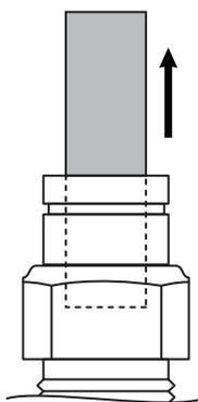
**4** To remove, push down collar and gently pull Air Tubing away.
